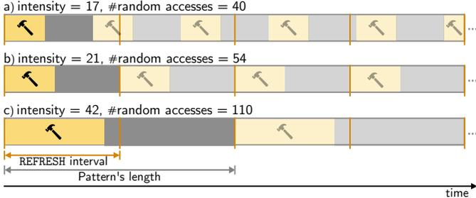
Fig. 7: **Regularity experiment.** Examples of tested patterns with different intensity and number of random accesses: a pattern smaller than (a) and of equal length to (b) a refresh interval, and (c) one covering two refresh intervals. Opaque regions show the pattern's repetition during execution.
