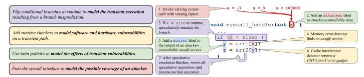
Fig. 2: Components used by our approach and how they interact to detect a PHT-USER-CACHE gadget in a system call handler.
